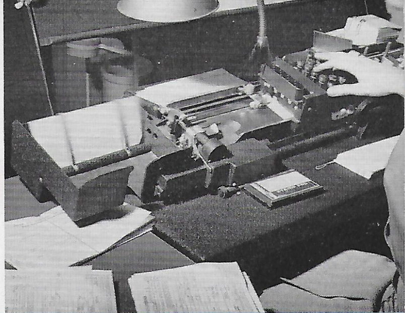
The numeric punch is used to transfer numerical data from delivery ticket to duplicate of proper master card. Below, Seattle's operators and machines are in action.
