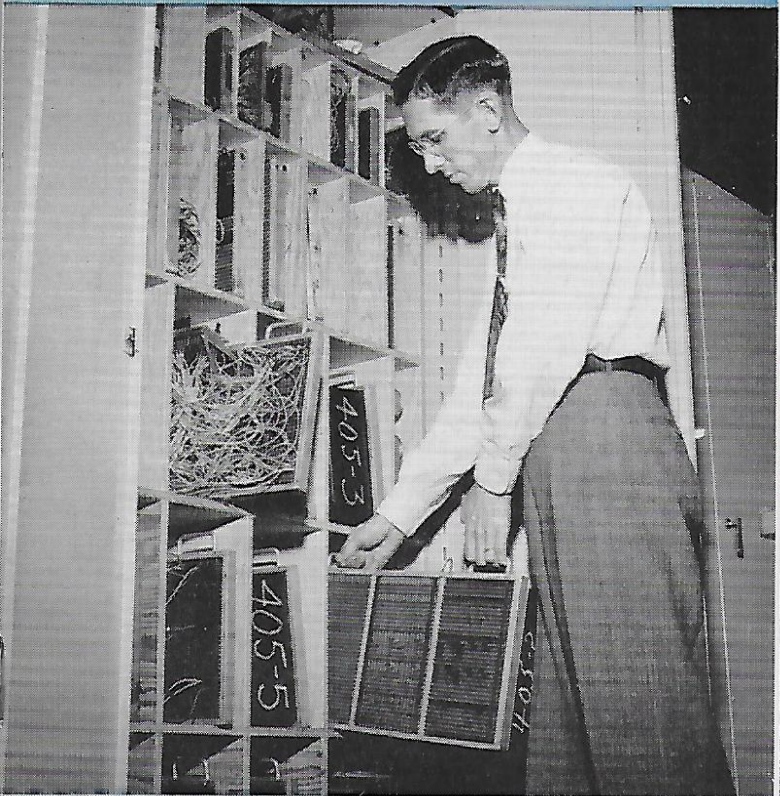
Plug-boards that control each machine's train of thought are stored in this cabinet for convenience—not for rest.
