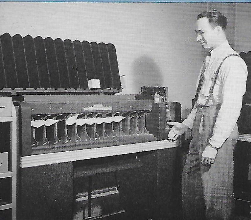
The electric card-operated sorting machine will sort cards into any desired sequence at about 600 a minute.
